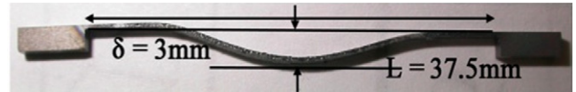
Fig. 6. ZrB 2 –SiC specimen after a creep experiment at 0.34 T magnetic flux density and 36 A current, corresponding to tensile stress of 20 MPa at 1750 °C, showing a creep deflection of 3 mm for about ~0.21% creep strain after 240 s.
