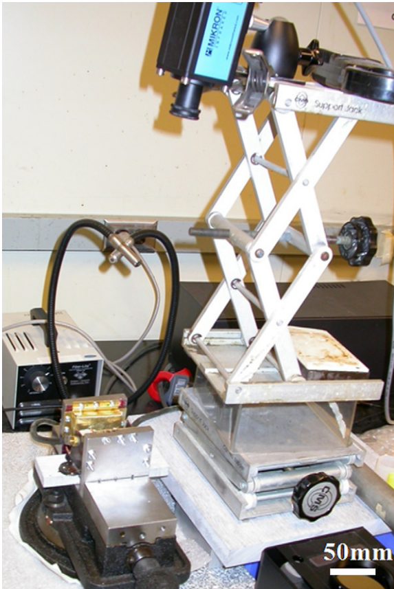
Fig. 4. Electro-Magnetic Mechanical Testing Apparatus (EMMA) system, showing the self-heating ribbon in the magnetic flux assembly on the benchtop, with the pyrometer above the hot ribbon.
